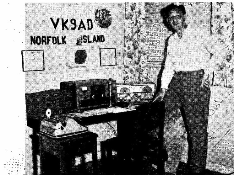
VK9AD is on Norfolk Is. in the South Pacific, at 28° 58' S., 168° 3' E. (Zone 32), the location for the trans-Pacific cable relay station of the Overseas Telecommunication Commission. VK9AD runs a Viking Valiant at 150w., with a Central Electronics SSB exciter, and his receiver is an SX-100; the aerial is a tri-band Quad, and he operates CW, AM and SSB on all bands. He complains of the very poor return on U.K. cards—he sends QSL's to G's, but simply does not have them back. VK9AD, who is one of those in distant parts who get "Short Wave Magazine" by airmail, has another six months to serve on Norfolk Is., but remarks that he will probably extend his stay for a further two years. So, if you owe him a card. . . .
