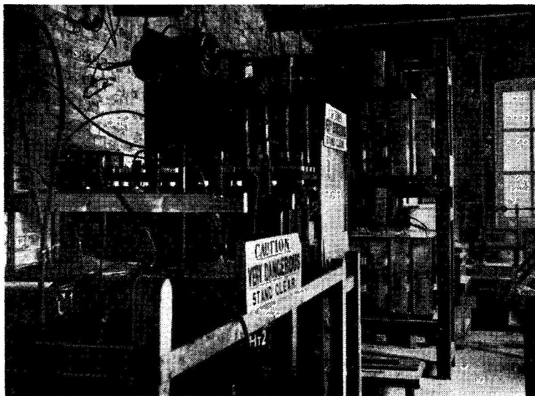
Marconi's spark transmitter at Poldhu, Cornwall, in December 1901, operating on a wavelength of "1200 to 1800 metres, not known exactly." The voltage across the spark-gap (right background) was 20,000v. and the transmitter was rated at 25 kW. It was this transmitter that put the first signal across the Atlantic, on December 12, 1901. (Photograph courtesy Marconi International Marine Communication Co., Ltd.)
