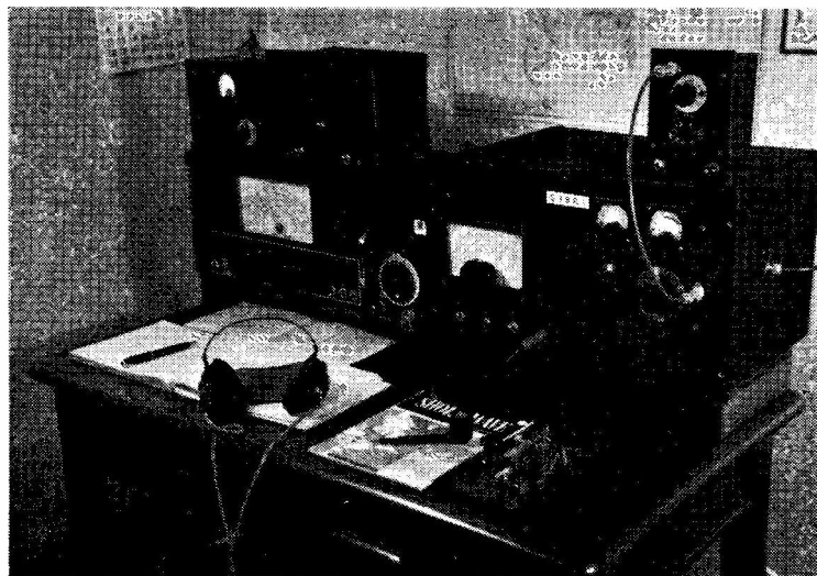
G3BCI of Bournemouth, Hants. was licensed in 1947, and is CW-only, running 30 watts to a home-built TVI-proofed transmitter, band switched for 14 and 21 mc. A separate QRP rig is used on 40 metres, and the receiver is an Eddystone S.640. Aerials are a dipole for 14 mc and a Zepp for the other bands.
